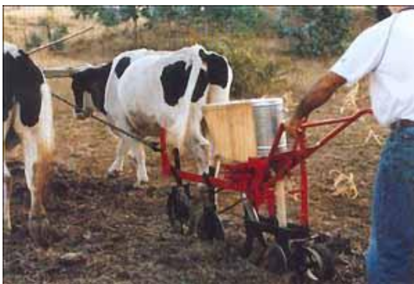
Fig. 13. Zero-tillage single planter with fertilizer attachment (A.D.Violic).
