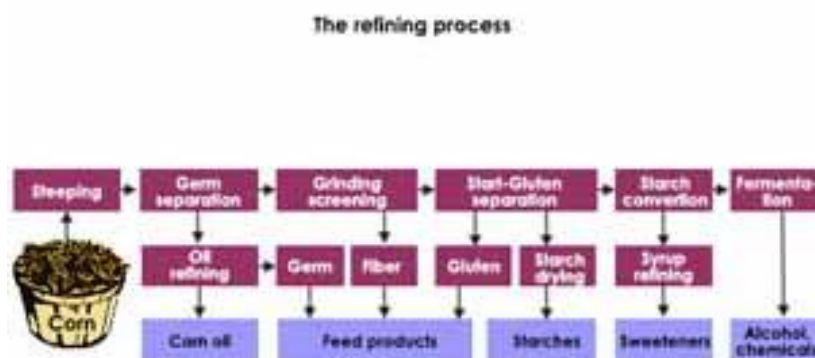
Fig. 11. Wet-milling Process flow diagram (Source: Corn Refining Assoc.)
