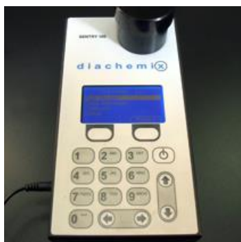
Figure 6: Portable fluorescence polarization reader Sentry® 100 for determination of various mycotoxins with assays from Diachemix Inc..
