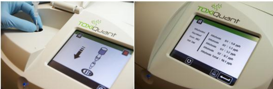
Figure 7: ToxiQuant, an instrument from ToxiMet Ltd, which automatically scans and analyses mycotoxins of a sample in a cartridge.
